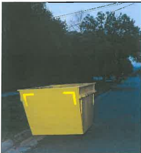
Retroreflective tape improves waste bin visibility.
