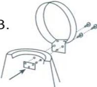
Place the lid on top of the green outer cone. Screw the hinge to the outer cone using three 10x5/8 self tapping screws and backplate as shown. When using these screws pre-drilled holes are not required.
