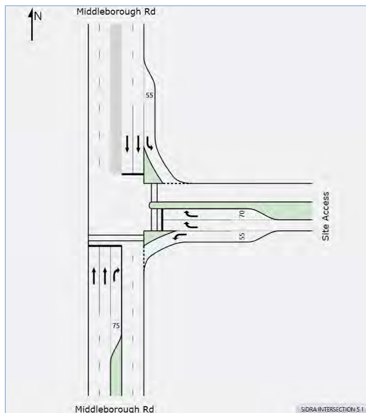
Figure 11: Middleborough Rd / Link Rd Proposed Intersection Configuration
