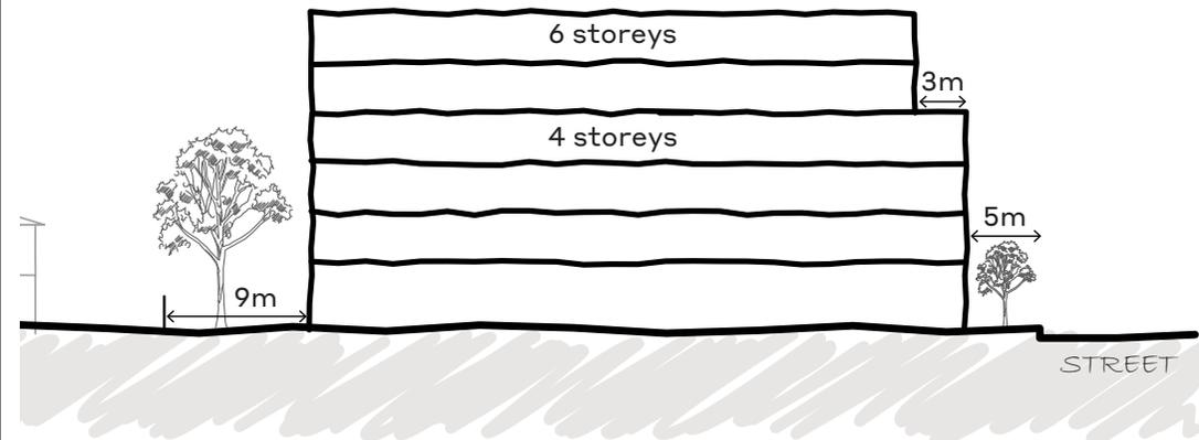
Side Elevation - Proposed Front and Rear Setback Standards
