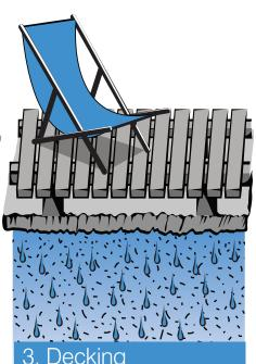
Unmade ground below, or with permeable treatment.
