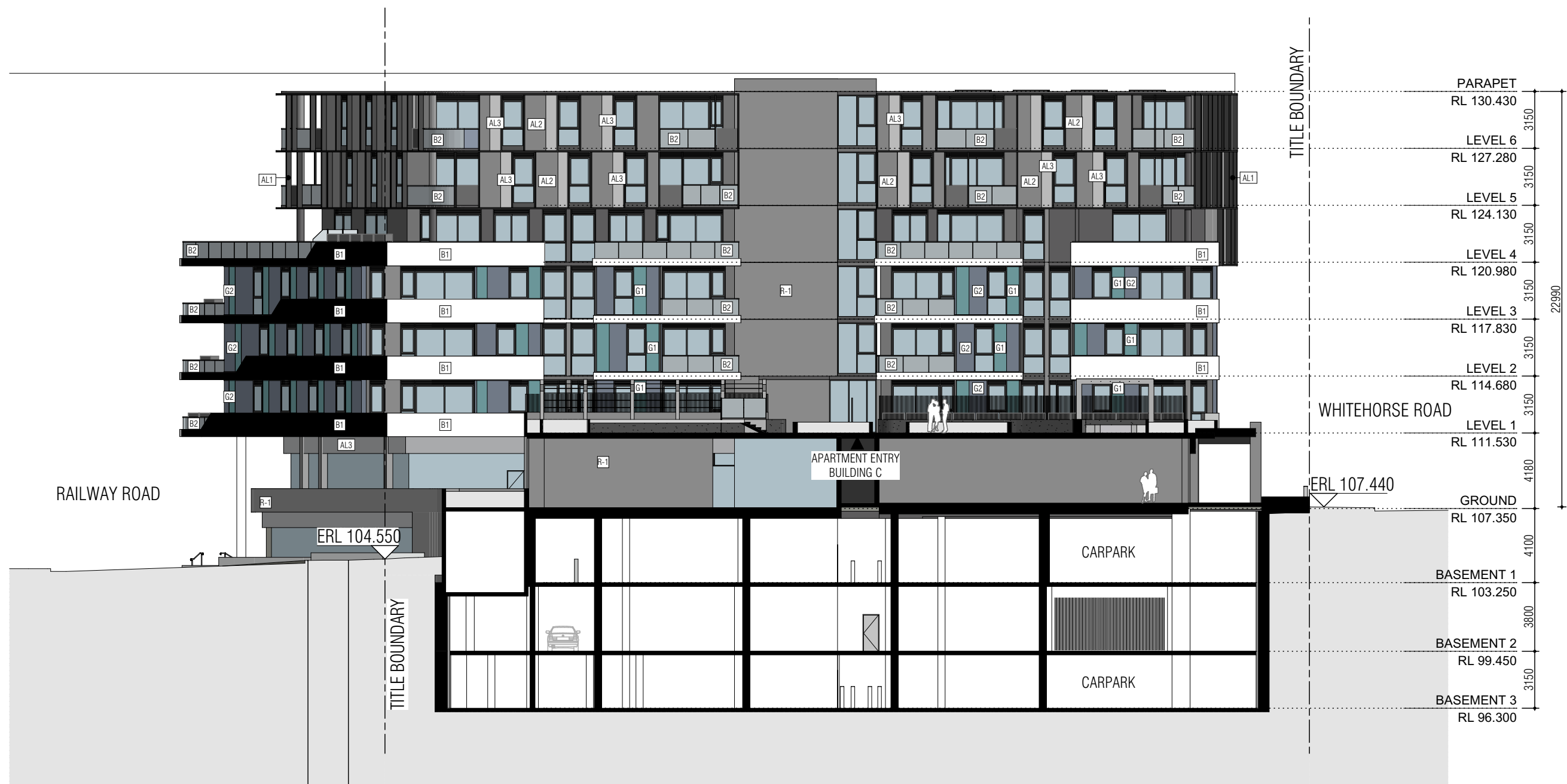
SECTION G - EAST ELEVATION - BUILDING C
