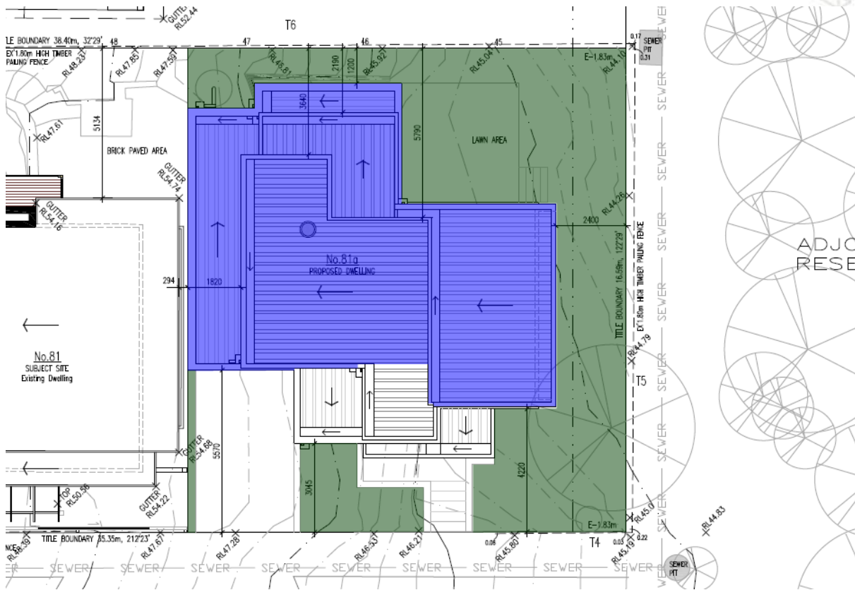
Figure 3: Roof catchment area for new dwelling to RWT (blue) and permeable areas (green).
