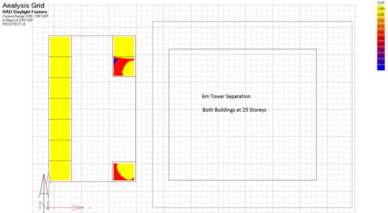
FIGURE 10: DAYLIGHT MODELLING RESULTS FOR EAST FACING BEDROOMS IN THE PROPOSED 874-878 WHITEHORSE ROAD HOTEL (25 STOREY TOWERS 6M TOWER SEPARATION).
