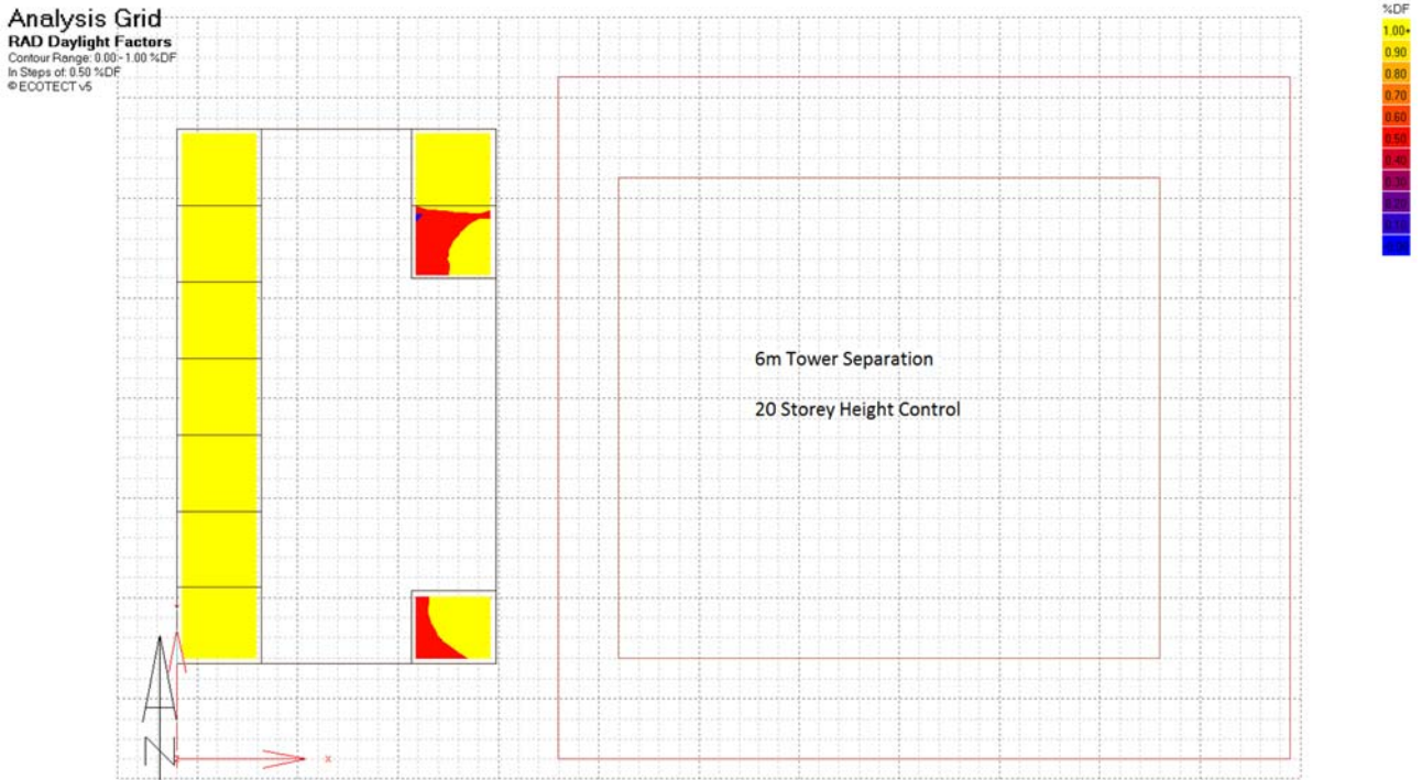
FIGURE 4: DAYLIGHT MODELLING RESULTS FOR EAST FACING BEDROOMS IN THE PROPOSED 874-878 WHITEHORSE ROAD HOTEL (20 STOREY TOWERS 6M TOWER SEPARATION).
